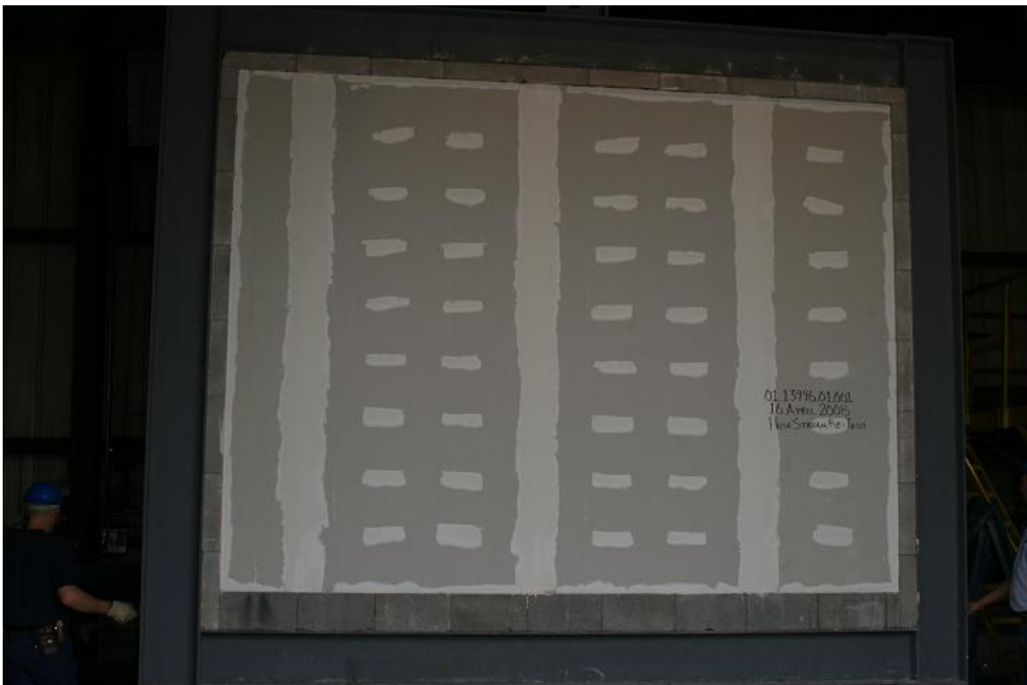
Figure B- 8. Unexposed Face of Hose Stream Test Wall prior to Furnace Exposure.
