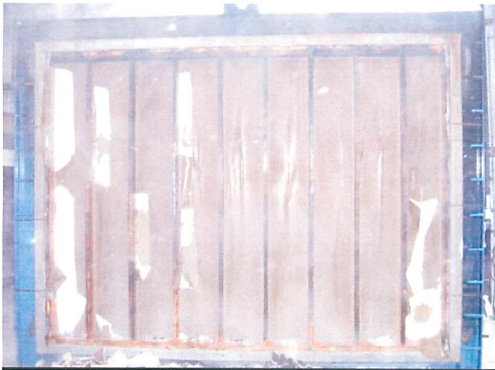
Figure A-8. Exposed Side of Hose Stream Retest Immediately After Hose Stream Test.
